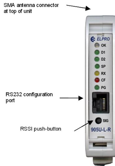
The LEDs on the front panel indicate the unit status:
